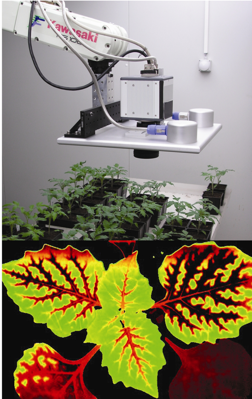
LED Induced Chlorophyll Fluorescence Transient Imager
