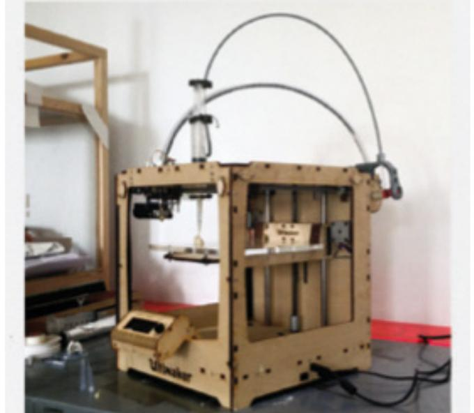
3D printing allows you to transform digital designed objects into physical objects. By modifying a conventional plastic printer into a bioprinter, a whole new range of materials can be used. Glucose scaffolds or even bacterial and fungi mediums. Your designs will finally truly come to life!
