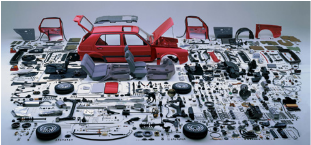
An example of a product (an automobile) broken-down into its individual components. (Image source: http://www.autohouston.net )
