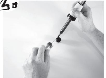
Place the MQ4 sensor down with the feet up and the sticker on the top. Solder the red wire from the battery holder to all the left feet.
