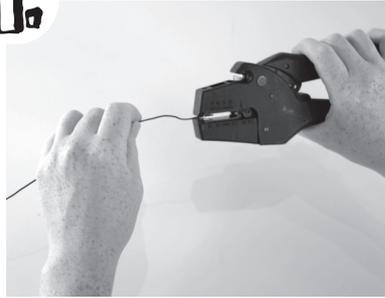
Cut one blue wire and two black wires and strip the ends. Also strip the ends of the wires on the battery holder.
