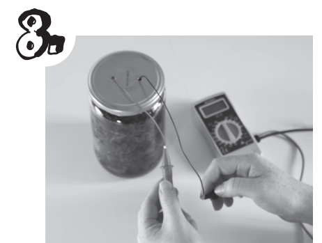
8. Microbes are so small that you can't see them. But if you get a lot of microbes together, they produce electric currents you can read with the voltmeter. TIP: Wait a day to get microbe levels up. More Volts means more active microbes in the ground.
