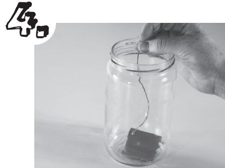
4. Place the copper plate on the bottom of the glass jar and drape the wire over the lip of the jar.
