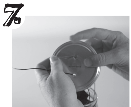
7. Make two holes in the jar lid, pull the wires through, and gently close the jar. Now connect the voltmeter cables to these two wires.
