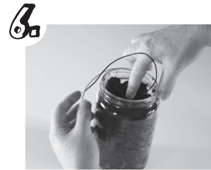
6. Now insert the screws into the soil and cover them with a final scoop of dirt.
