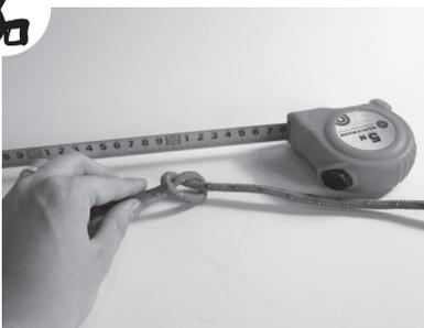
Measure 10 cm away from the LP along the rope. Tie a knot here. Make another knot every 10 cm until the end of the rope.
