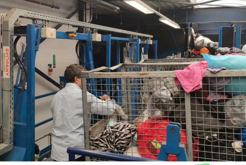
**Above:** Textile waste must be sorted by colour and composition before recycling. Sorting is usually done manually, but technological advancements mean that automatic sorting will be more prevalent in the future.
