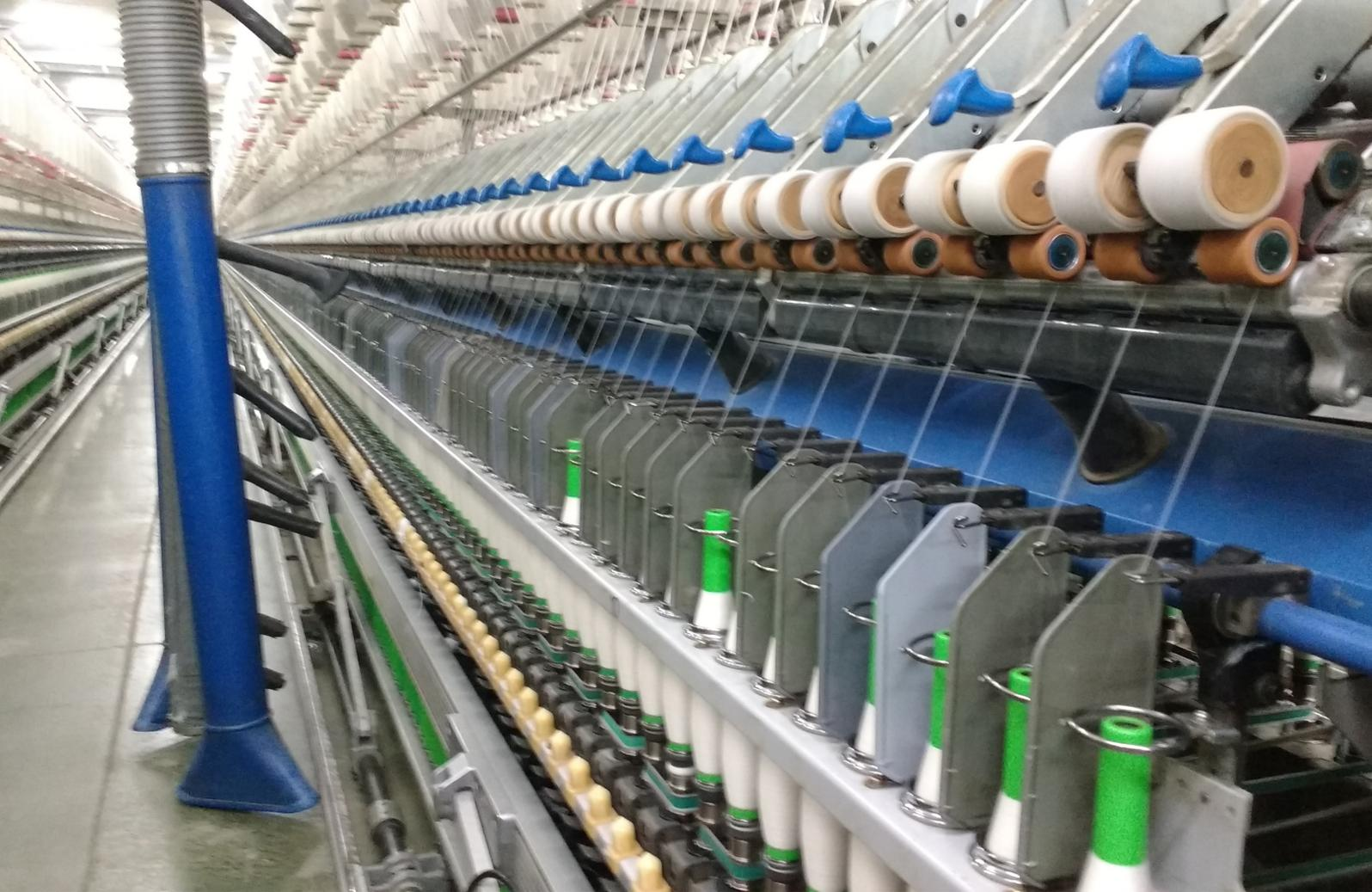
**Above:** Spinning is one of the most complex and demanding parts of the textile production chain. Spinning involves bringing the staple fibres in close contact with each other, twisting them around each other while simultaneously stretching the fibre bundle.
