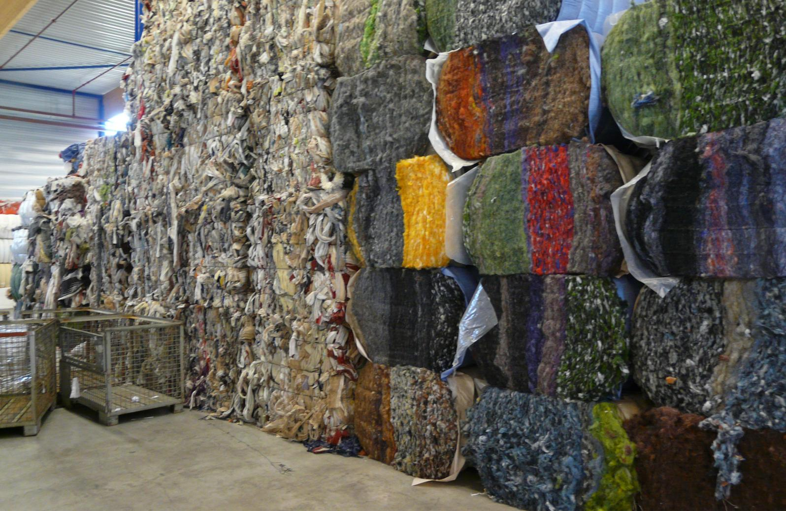
**Above:** Thermoplastic textile waste must be sorted prior to recycling by extrusion. Sorting materials based on colour will result in a more homogeneous colour, but colour variations often occur.
