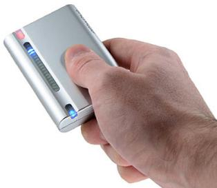
The Emwave works quite similar to the StressEraser. By means of a infrared sensor the Emwave measures blood saturation in finger tissue. From this data it computes pulse and HRV. When the HRV is irregular, Emwave will indicate this. It also shows a breathing pattern to regulate the HRV, using the blue led bar.
