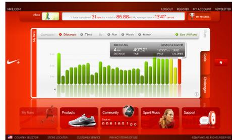
The Nike + Sensor measures pace, distance, time and calories burned. This information is wireless transmitted to either a Nike+ SportBand or a iPod/iPhone. This information can be uploaded to a website to track progress and achievements.
