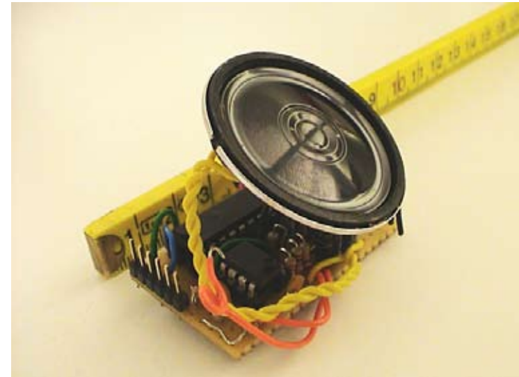
Meshy board - de elektronica en luidspreker die in Meshy wordt verwerkt/ Meshy board - the electronics and speaker that will be incorporated in Meshy.
