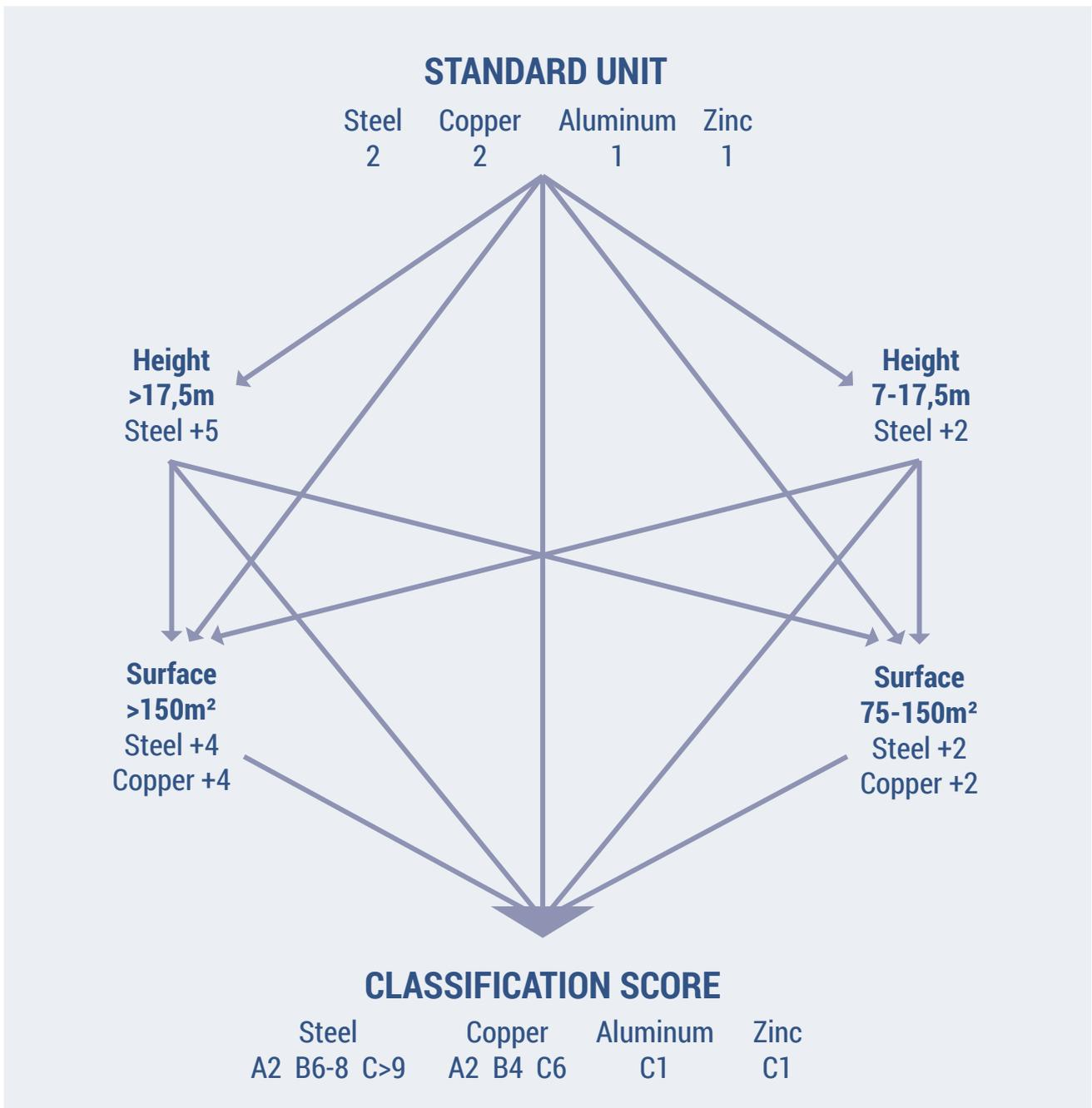
Figure 1: Flow-chart for categorizing housing units into metal content classifications
